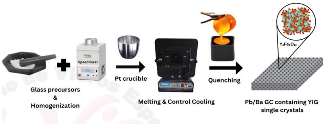
Figure 22. Schematic of YIG single-crystal synthesis in glass-ceramics.
