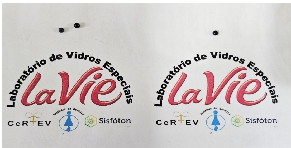
Figure A-4. Bulk YIG samples were synthesized using a containerless processing technique (levitation melting) for MO measurements.
