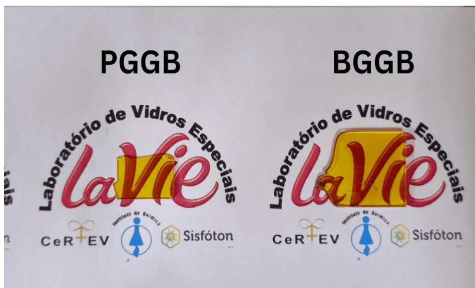
Figure 26. The blank glasses for PbO (PGGB) and BaO-based systems (BGGB).
