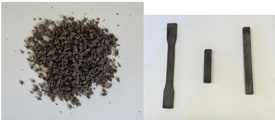
Figure 1. Composites pellets ready for injection molding and the samples used for testing.
