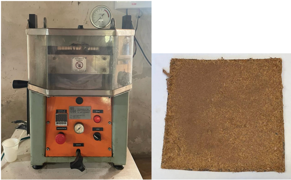
Figure 2. Press used for the boards, with hot and cold plate. The binderless coir board.
