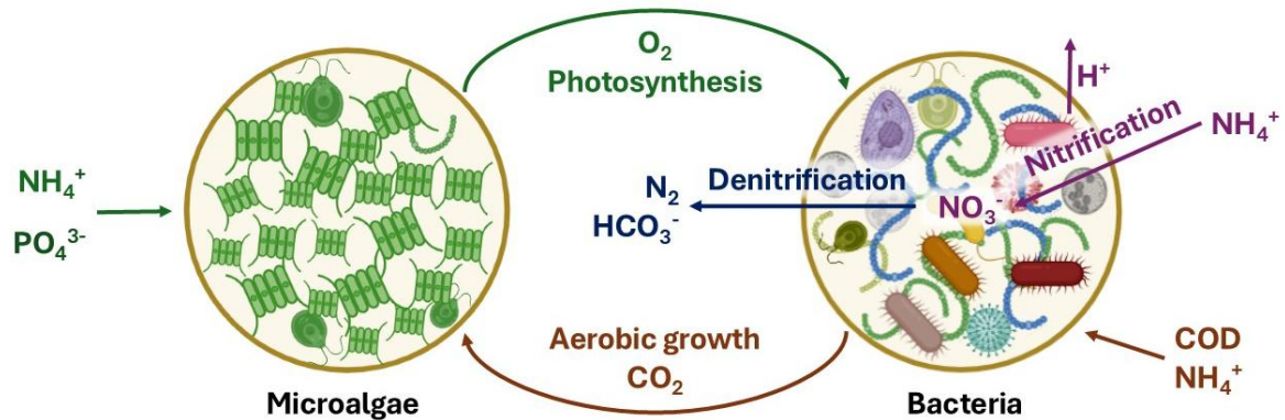
Figure 5: Schematic representation of the synergistic interactions in a microalgal-bacterial system. The diagram illustrates photosynthesis (green), aerobic growth (brown), nitrification (purple) and denitrification (blue) processes. Drawing from Biorender.
