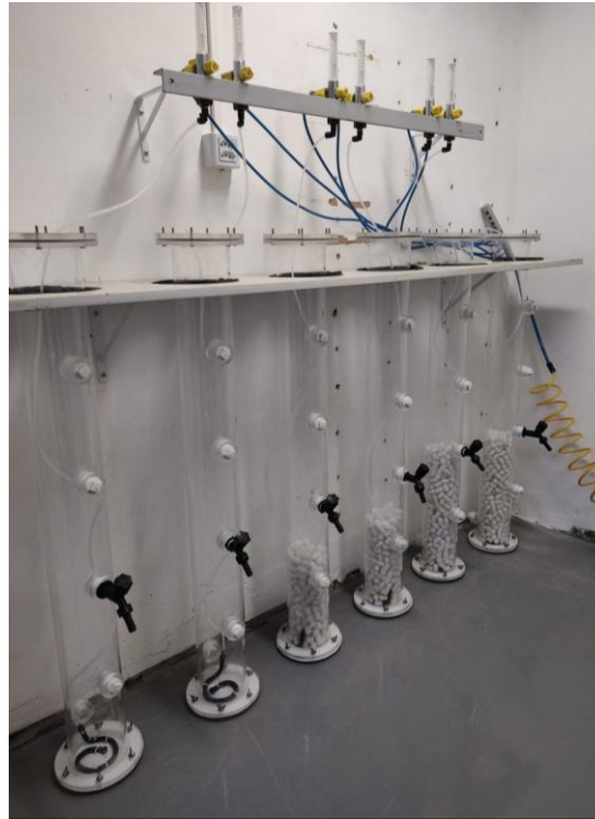
Figure 10: Column photobioreactors with and without support media.
