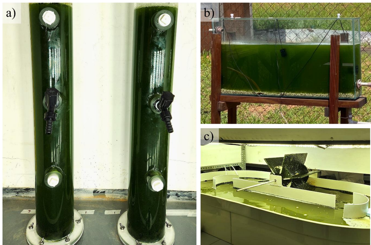
Figure 7: Photographs of closed microalgae cultivation systems installed at UNESP - Bauru: (a) column photobioreactors and (b) flat panel; and open system installed at the Institute of Sustainable Processes, University of Valladolid (c) high-rate algal ponds (HRAP).
