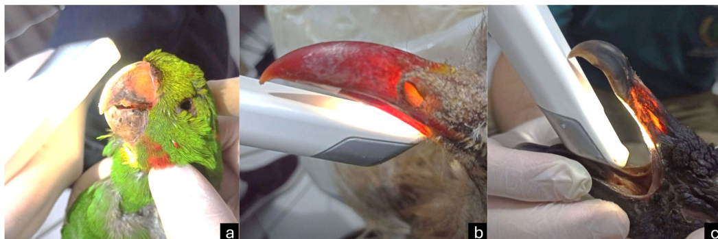
Figure 4. Scanning of parakeet (a), red-legged seriema (b), and black vulture (c) beaks with dental intraoral scanner.
