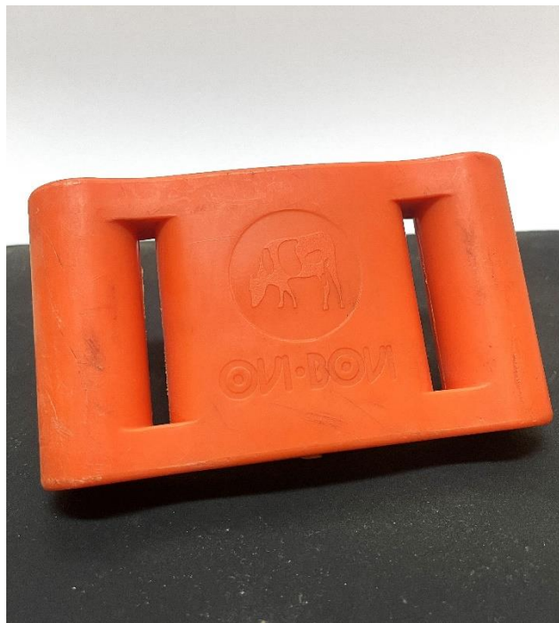
Figure 1. Ovi-bovi ® tag which contains an accelerometer device inside the shell.
