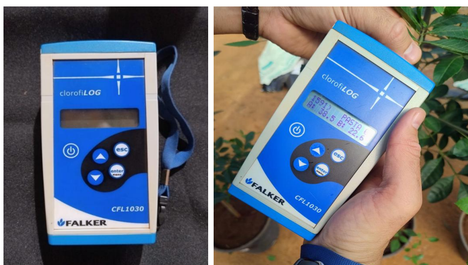
Fig. 87 and 88. ClorofiLOG FALKER, model CFL 1030 and leaf chlorophyll index measurement.
