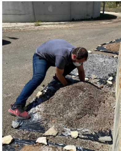
Fig. 20. Daily manual stirring of the mixtures during the stabilization period.
