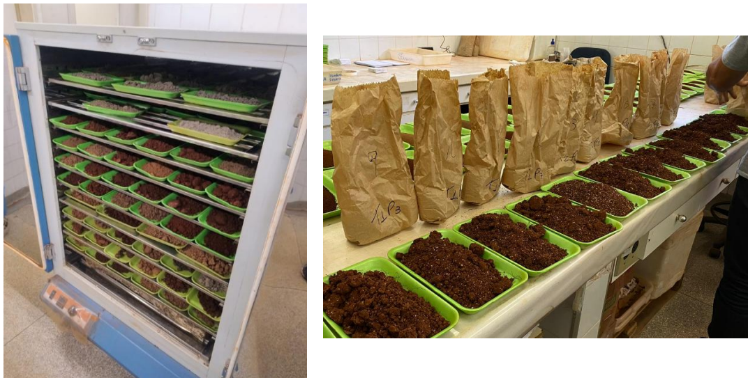
Fig. 76 and 77. Samples inside the forced-air drying oven and then on the bench for further sieving.
