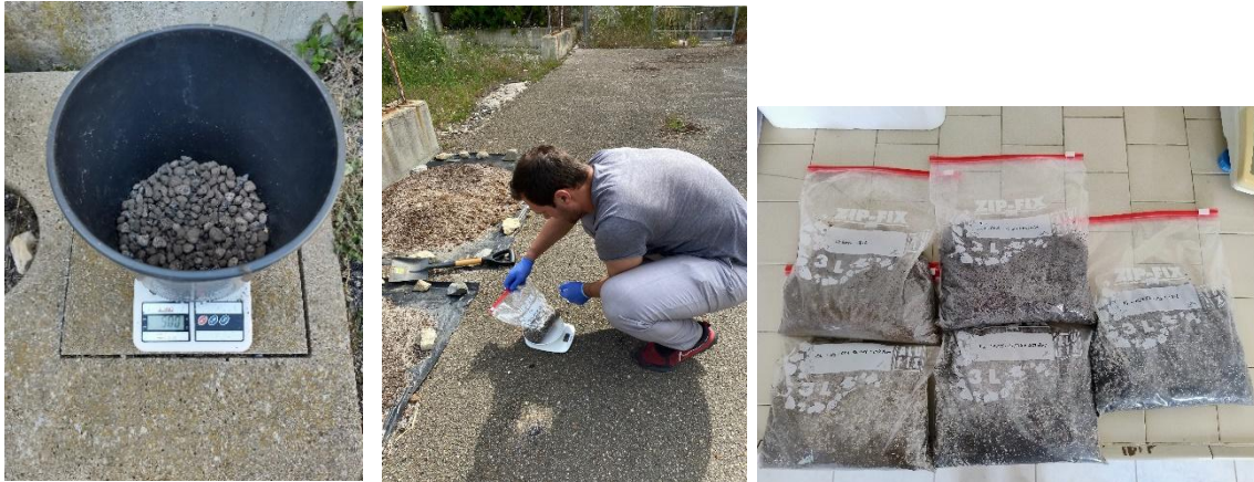
Fig. 28, 29 and 30. Addition of expanded clay to the bottom of the pots (left); weighing of substrate samples by treatment (center); identification and packaging of samples for sending to laboratories (right).
