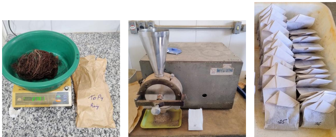
Fig. 97, 98 and 99. Weighing of the dry root (left); grinder used for initial grinding of the roots (center); samples prepared for sending to the laboratory for nutritional analysis (right).
