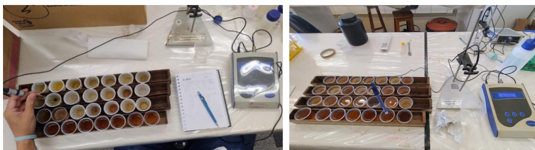
Fig. 85 and 86. pH reading (left); electrical conductivity measurement (right).
