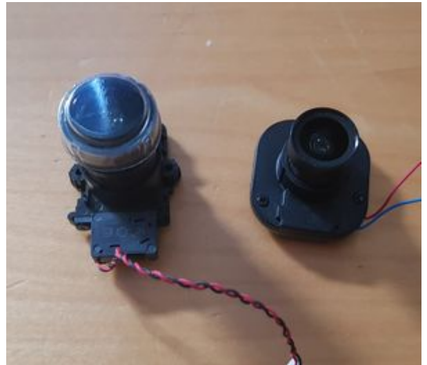
Two sorts of lens holder with day/night filters
