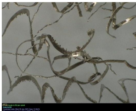
a_p = 0,1\text{mm} . cavaco helicoidal longo
