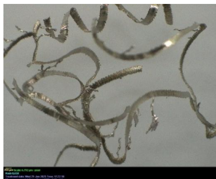
a_p = 0,2\text{mm} . cavaco helicoidal longo
