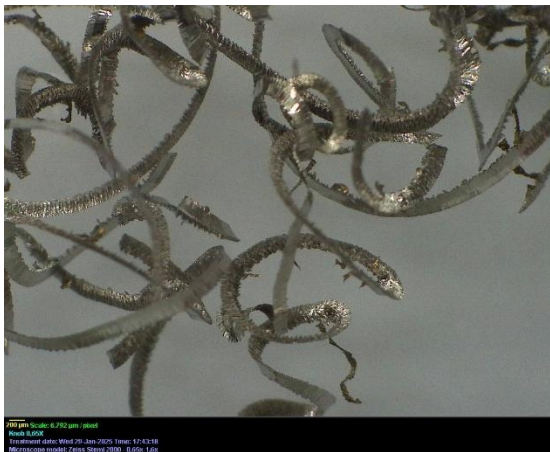
a_p = 0,1\text{mm} . cavaco helicoidal longo
