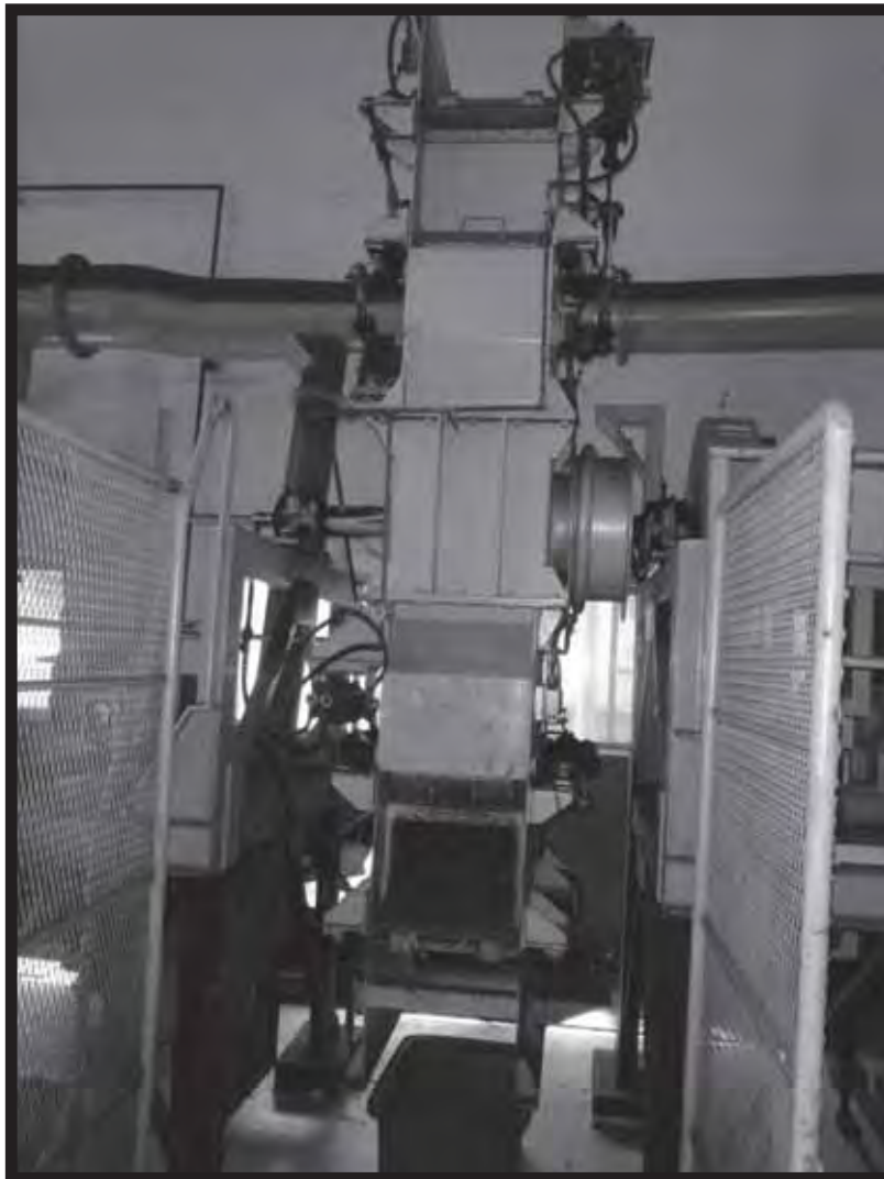
Figura 6.6 – Shatter Test conforme norma NBR 10633
