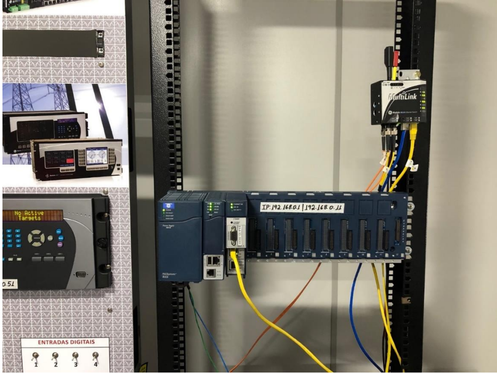
Figura 18 - CLP GE IP Rx3i e Switch GE ML600.
