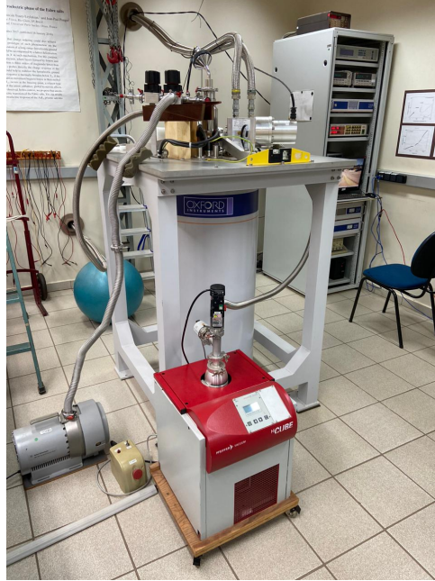
Fig. 19 – Front view of the Teslatron-PT with both scroll and the turbo pump connected to the system.
