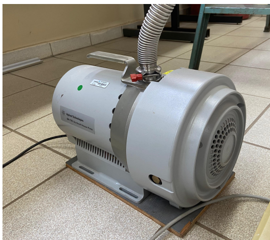
Fig. 33 – Lateral view of the SH-110 scroll dry pump present in the Solid Physics State Laboratory.
