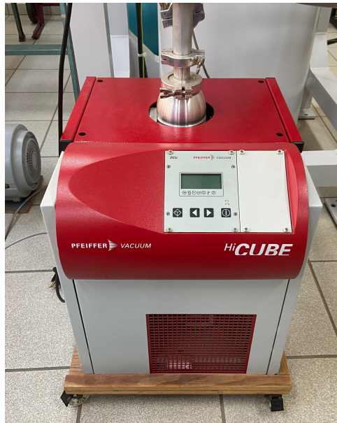
Fig. 35 – Front view of the HiCube 80 classic turbo pump present in the Solid State Physics Laboratory.
