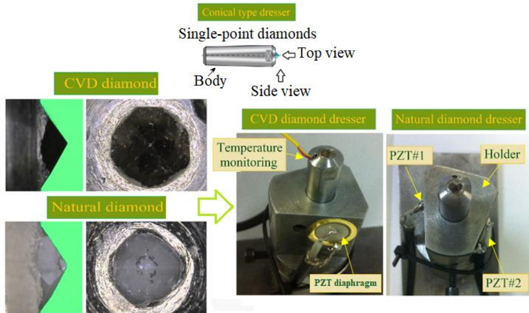
Figure 34- Experimental test case #1: stationary conical single-point dressers, top and side views of both diamond tips, PZT diaphragms attached to the tool holder, and temperature monitoring procedure
