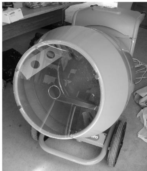
Figure 3.3. Extraction equipment using a concrete mixer developed.
