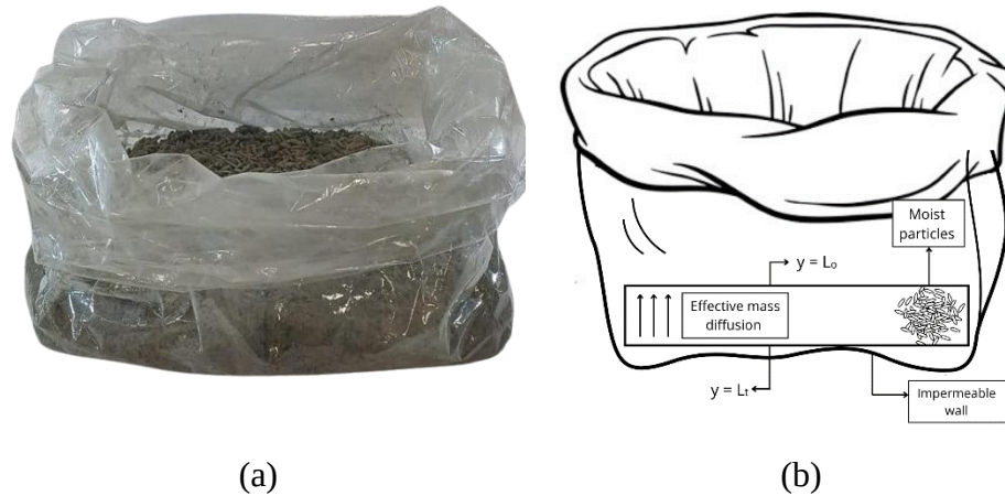
Figure 4.2. (a) Plastic packaging during the drying process; (b) Diagram of mass transfer on a flat plate with the conditions adopted in the mathematical model.
