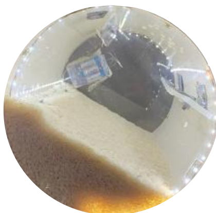
Figure 7.6. Rotating drum used to establish the movement regime of raw rice particles.
