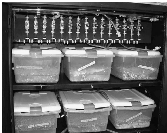
Figure 3.2. Adapted plastic boxes for faster drying of conidiated rice.
