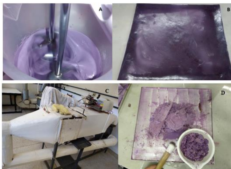
Figure 3.2 - Production of foam containing the juice (A), foam placed on the tray (B) for the subsequent drying stage (C) and final product being macerated (D).
