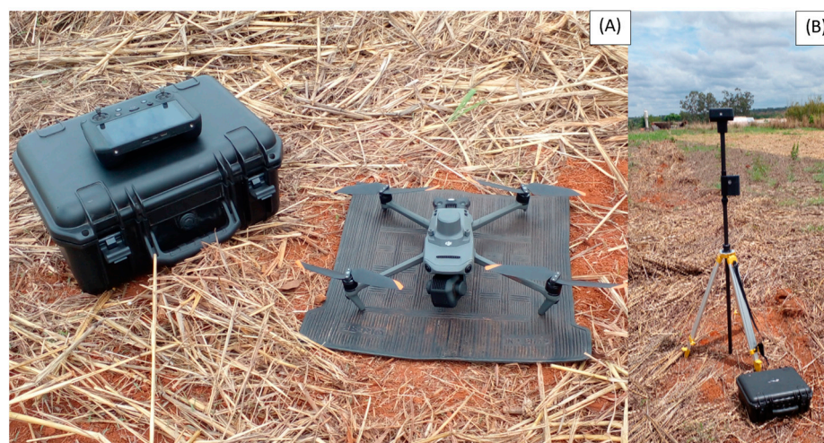
Figure 3. Equipment used for image acquisition and georeferencing. (A) DJI Mavic 3 Multispectral with controller and case. (B) GNSS DJI D-RTK2 base station for precise positioning.
