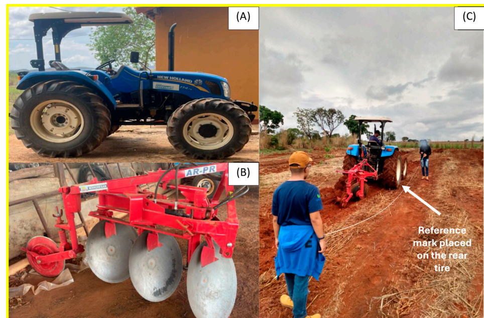
Figure 1. (A) New Holland TT4.75 tractor with ballast configuration (front weights: 240 kg; rear water tanks: 270 L/tire). (B) Marchesan AR-PR reversible plow with 710 mm discs and adjustable arms. (C) Slip test procedure.
