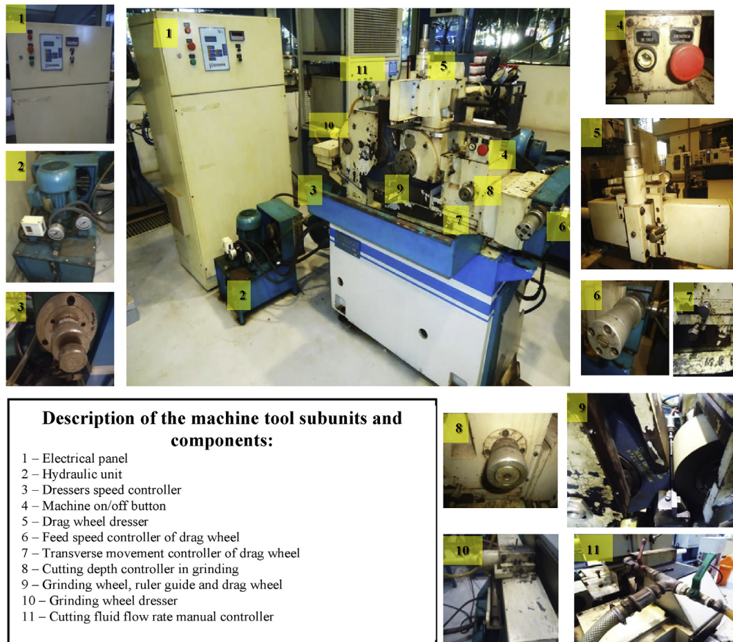
Fig. 12. Overview of the centerless grinding machine sited at LAPRAS-EESC-USP.
