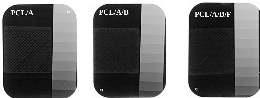
Figura 59. Fotos radiográficas das amostras \text{PCL}:\text{La}_{20}\text{OAP} , \text{PCL}:\text{La}_{20}\text{OAP}:\text{BV} e \text{PCL}:\text{La}_{20}\text{OAP}:\text{BV}:\text{FB} .
