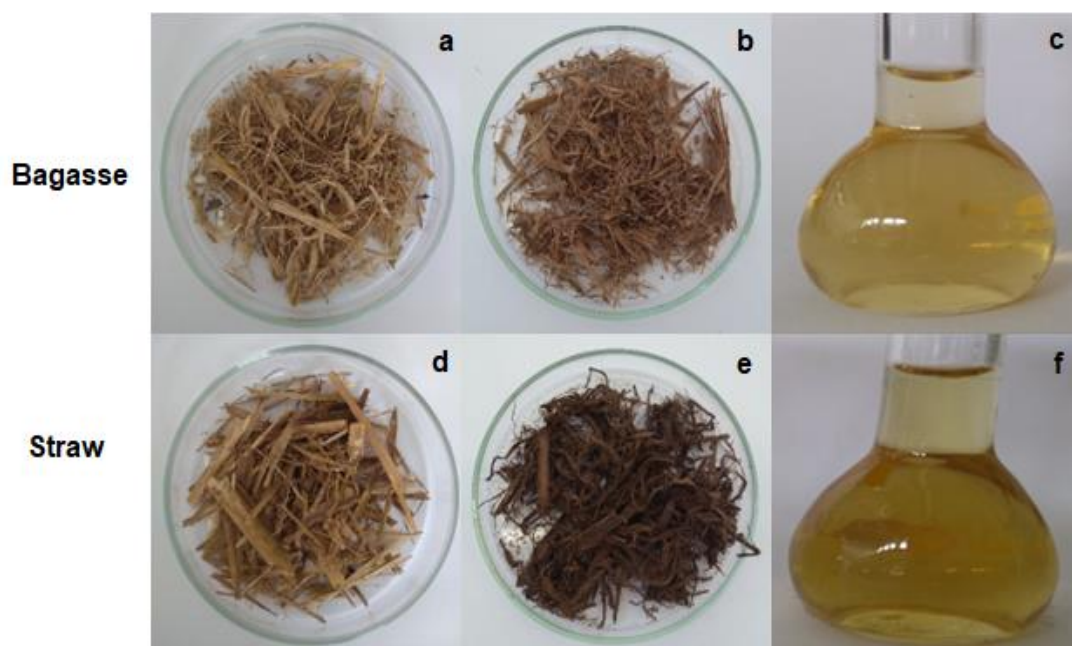
Figure 2.7. Untreated SB and SS (ad); Recovered solids after HP in SB and SS under optimized conditions (be); HH from SB and SS after HP under optimized conditions (cf), respectively
