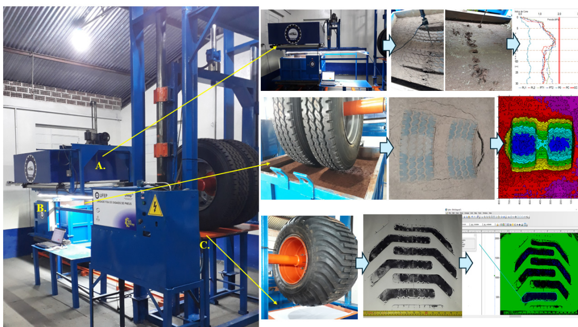
Figure 1. Static tire test unit (STTU). (A) Scanner system and soil penetration resistance (SPR); (B) soil bin (deformable surface); (C) steel desk (rigid surface).
