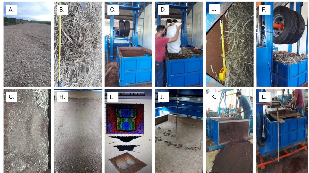
Figure 2. Procedures for assembling soil bins under control conditions to simulate agricultural soil—Nempa/Botucatu laboratory. (A) Selection of plant material in sugarcane commercial crops (straw); (B) quantification of straw, biomass water content and distribution over the soil; (C) assembling the soil bin with controlled density and moisture; (D) distribution of cover over the soil in different quantities; (E) assessment of cover and removal of a sample of the initial soil penetration resistance from the soil bin; (F) application of load with the wheel on the soil bin; (G) removal of straw to assess soil deformation; (H) soil scanner (Lidar) to assess footprint; (I) assembling 3D maps of each soil tank; (J) assessment of soil penetration resistance in a soil bin transect; (K) unloading the soil tank; (L) standardization of moisture, sieving and loading the tank for a new test cycle.
