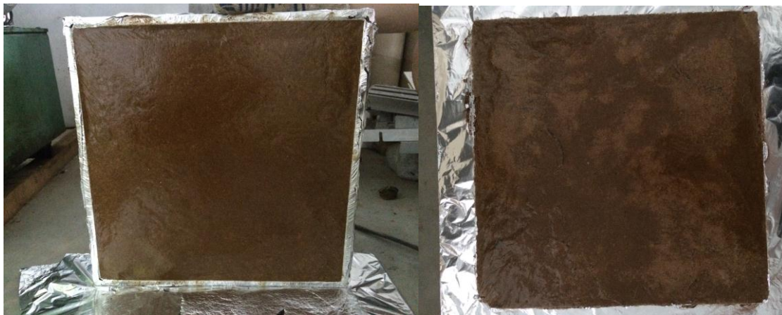
Figura 38: a) Painel de 50PP30CA10FC; b) Painel de 30PP45CA25FC
