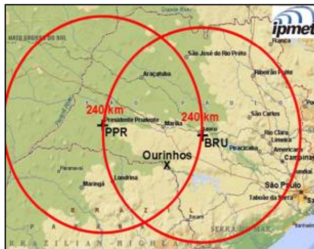
Figure 1: IPMet's S-band radars in Bauru (BRU) and Presidente Prudente (PPR) with the quantitative radar ranges of 240 km..
