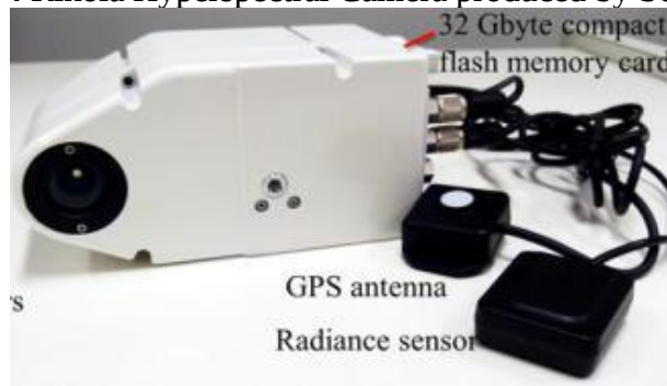
Figure 4 Rikola Hyperspectral Camera produced by Senop Ltda
