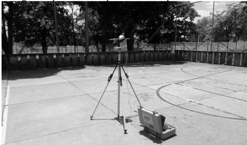
Figure 7 Operation of the spectrometer to acquire irradiance data.
