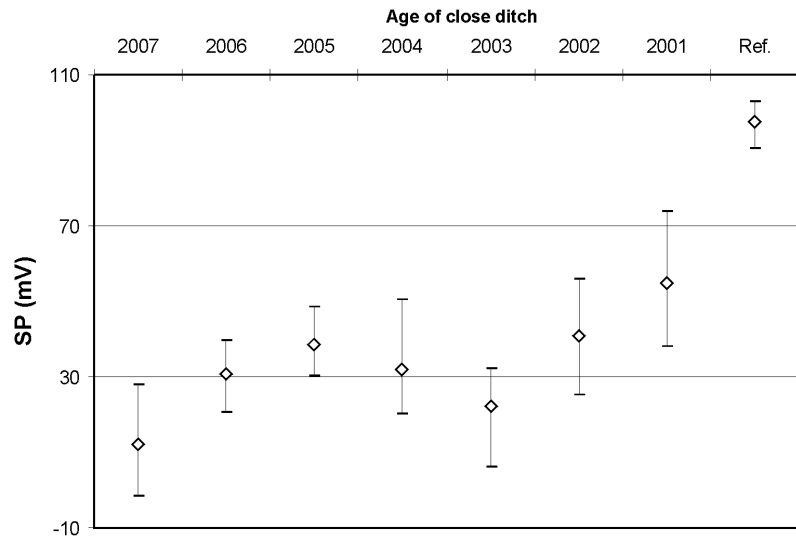
Figure 4. Mean and extreme values of SP for the second stage surveys.
