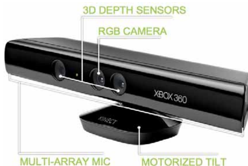
Figure 16 - Microsoft Kinect sensor system (JANCKE, 2011)
