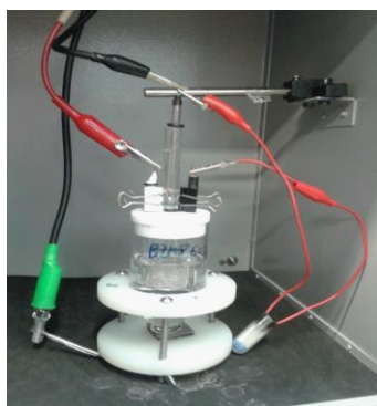
Fig. 7 .Electrochemical cell in a faraday cage used for EIS measurements.
