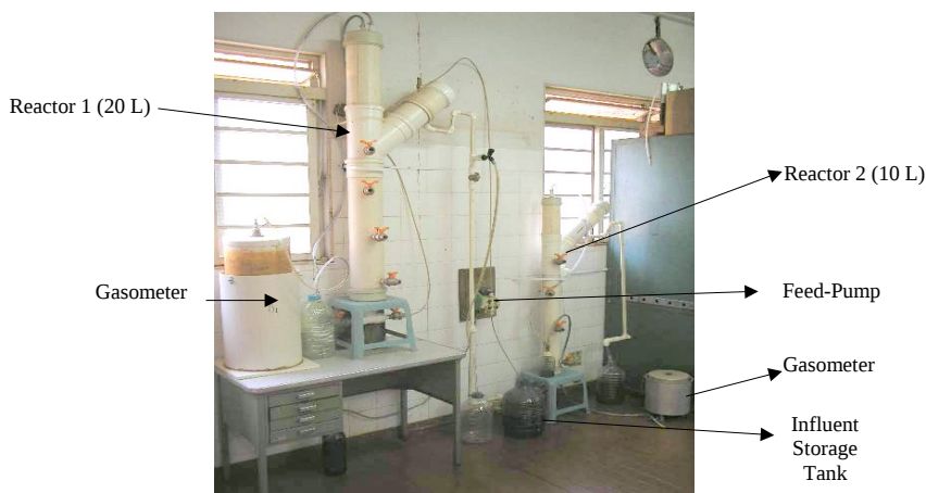
Figure 1. Upflow Anaerobic Sludge Blanket (UASB) in two-stage system, feed-pump, influent tank storage and gasometers.
