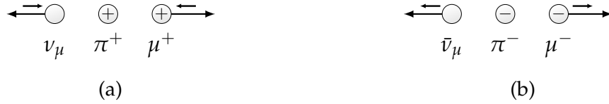
Figure 4.1: Pion decay, \pi^\pm \rightarrow \mu^\pm + \nu_\mu (\bar{\nu}_\mu) , in the pion rest frame. The long arrow represents the momentum of the particle and the short one, which is above the long arrow, represents the spin of the particle.
