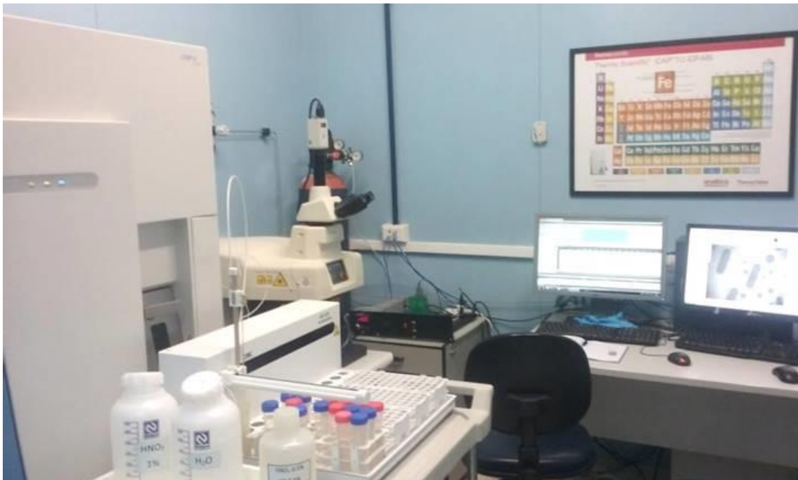
Figure 4.3 – New Wave UP-213A/F laser ablation system (center-left) coupled to a Thermo iCAP Q quadrupole ICP-MS (left) at the Institute of Geosciences, University of São Paulo (USP).
