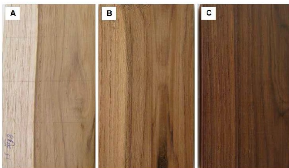
Figura 10 - Madeira de Tectona grandis ; (A) madeira original, (B) tratada a 180°C e (C) tratada a 200°C.
