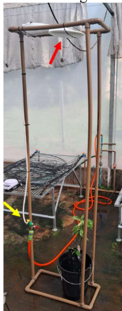
Figure 8 - Washing system used on adhesion test experiments. In red the droplet disperser, in yellow the valve used to regulate the water flow.
