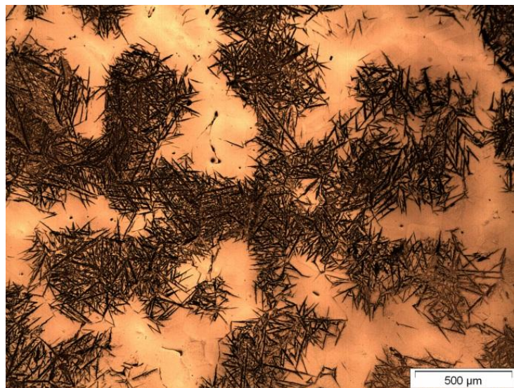
Figura 26 – Amostra homogeneizada – 1150°C / 8 h – Nital
