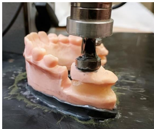
Figure 5. 3D resin model fixed onto the desk top table of the orthodontics force tester machine.
