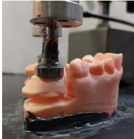
Figure 7. Second molars completely separated from the 3D resin model, which is glued onto the OFT desk top, but attached to the OFT machine load cell.
