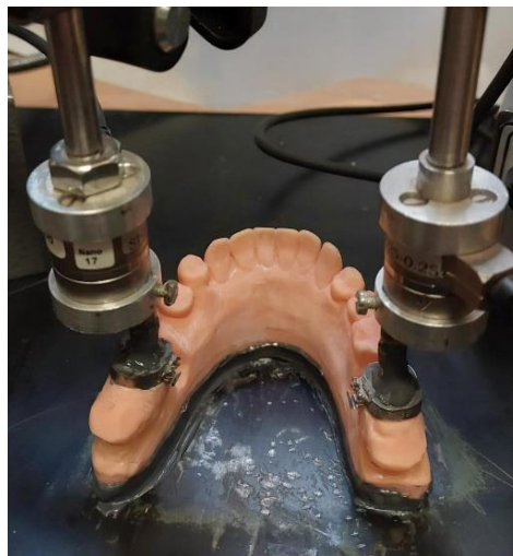
Figure 6. The two load cells positioned and glued to the second molars, which were previously separated from the 3D resin and repositioned back with.
