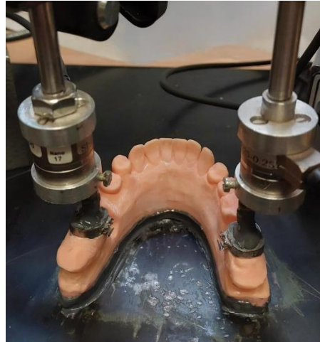
Figure 6. The two load cells positioned and glued to the second molars, which were previously separated from the 3D resin and repositioned back with.
