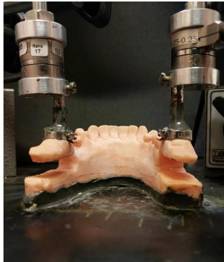
Figure 7. Second molars completely separated from the 3D resin model, which is glued onto the OFT desk top, but attached to the OFT machine load cell.
