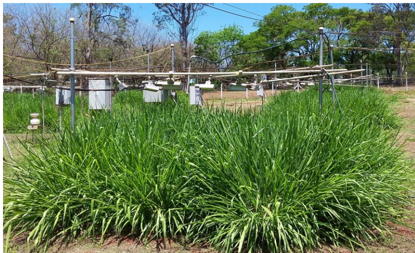
Figure 1. Temperature Free-Air Controlled Enhancement (T-FACE) Systems in guinea grass. Photo: Dilier Olivera Vicedo
