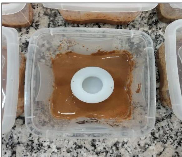
Figure 19: DGT device deployed in soil sample at 100 % water holding capacity (Gemeiner, 2020).
