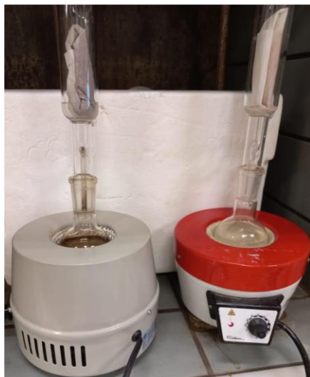
Figure 7. Soxhlet system for removal of analyte from mag-MIP Source: Author
