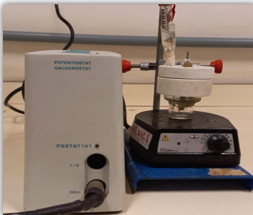
Figure 9. The photography depicts the batch electrochemical measurements that carried in electrochemical cell, which include typical three electrodes setup as well Source: Author
