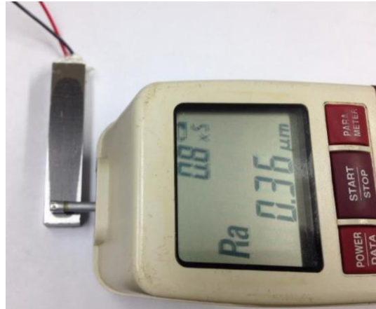
Figure 6 – Surface roughness measurement for the ABNT N2711 steel
