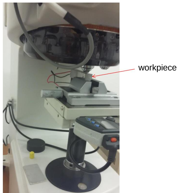
Figure 5 – Microhardness measurement for the ABNT N2711 steel
