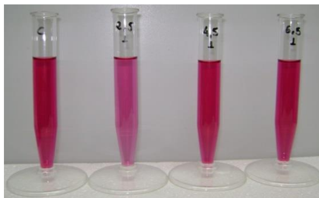
Figure 6 – Visual evaluation of DR75 solution in four different pH values, the control (c) with pH around 7.0 and the samples with pH 2.5, 4.5 and 6.5
