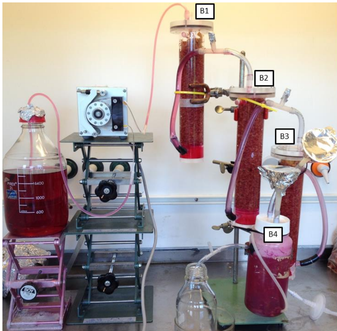
Figure 5 – Bioreactor B composed by the sequenced bioreactors B1, B2, B3 and B4 (aerobic)
