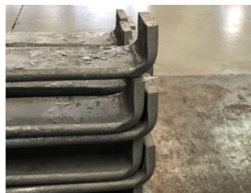
Figure 9 – Springs after fold. Source: Author.
