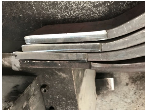
Figure 13 – Springs after face milling. Source: Author.
