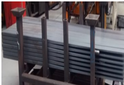
Figure 3 – Springs after parabolic lamination. Source: Author.
