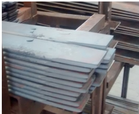
Figure 4 – Springs after conventional lamination. Source: Author.
