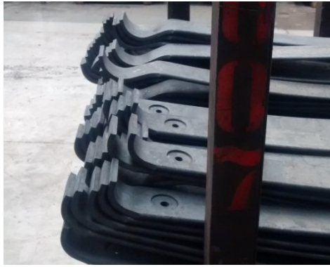
Figure 8 – Springs after semi-fold. Source: Author.
