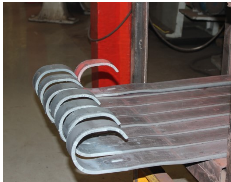
Figure 6 – Springs after second fold. Source: Author.
