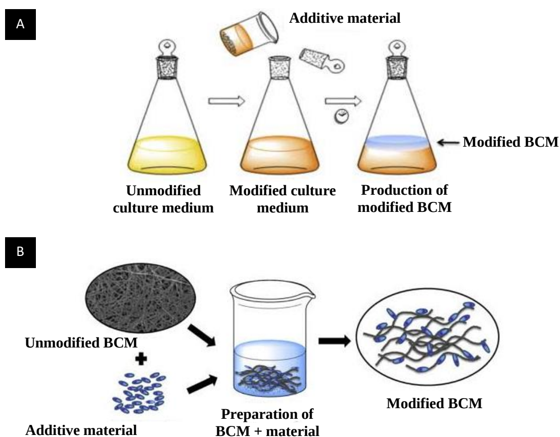
Figure 3 –Schematic representation of preparation of BCM modifications methods: (A) in situ and (B) post-grafting [5].
