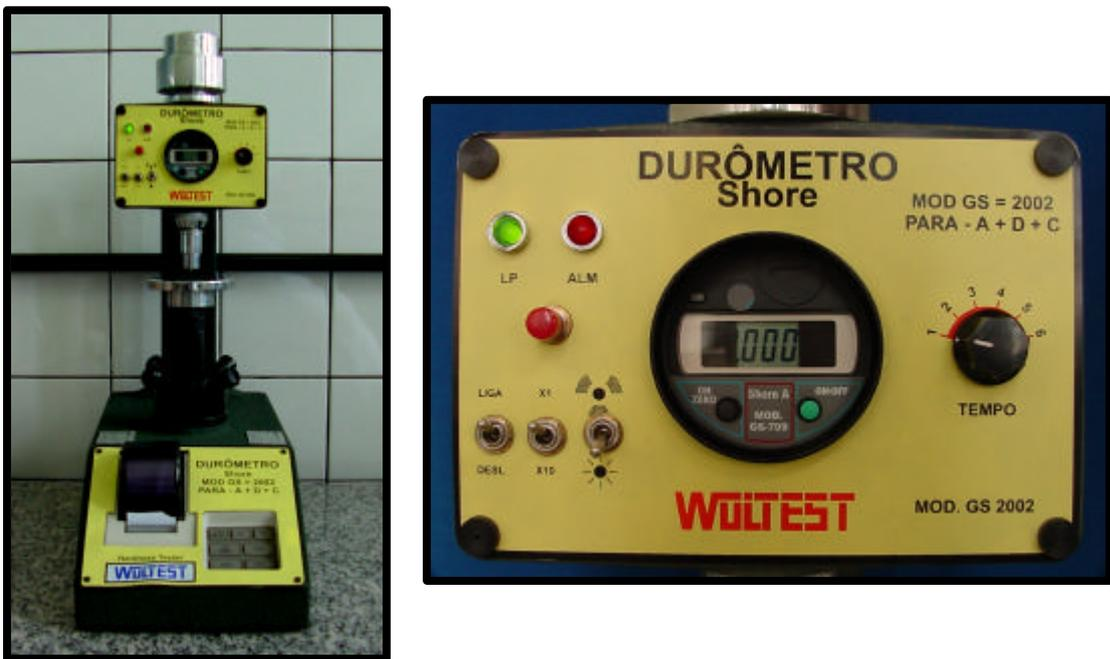
FIGURA 10 e 11: Durômetro Shore A e painel de controle
