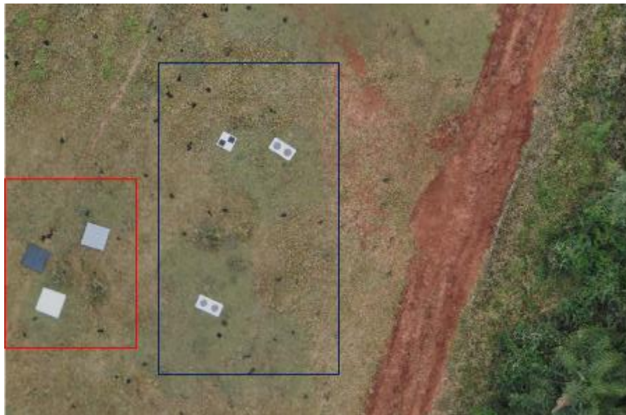
Figure 2 – Targets located near the overflow area. In red the radiometric targets, and in blue the GCPs targets.
