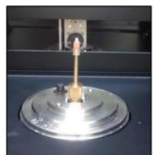
Blocos no interior do Micro-CT
