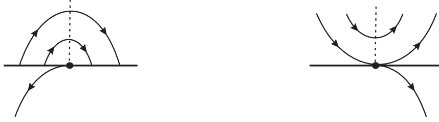
Figure 4.34: (Invisible) Fold – Cusp (of kind 1) Singularity. Figure 4.35: (Visible) Fold – Cusp (of kind 2) Singularity.
