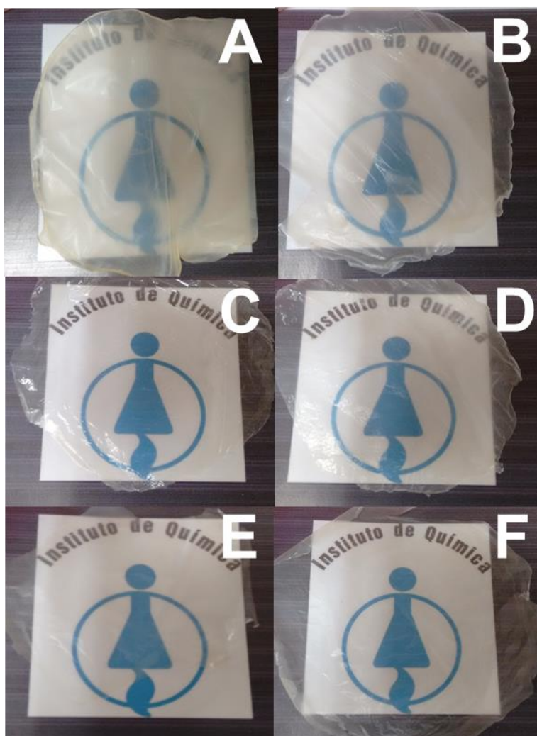
Figura 10. Filmes obtidos. CB pura (A), CB + 0,1% LP (B), CB + 0,25% LP (C), CB + 0,50% LP (D), CB + 0,75% LP (E), CB + 1,0% LP (F).
