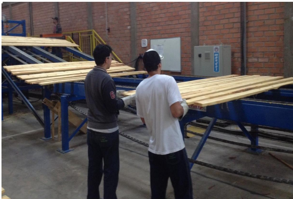
Figure 19 – Visual classification of Pinus boards
