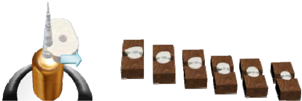
FIGURE 2: Trimmed procedure in each slice by an ultra-fine diamond bur mounted in a high speed hand piece with water coolant.
