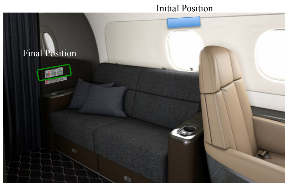
Figure 31 - Seat Occupancy Placard Installation Position
