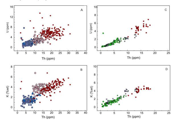
**Figure 16.** Th (ppm) vs. K (% wt), and U (ppm) obtained by gamma-ray spectrometry in this study (A and B) and geochemical data (C and D) from of Marques (1988) and Marques et al. (1989). Legend: as Figure 15 (for A and B) and Figure 13 (for C and D).
