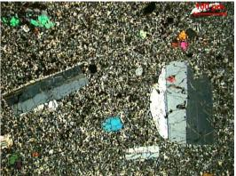
**Figure 8.** Photomicrography under crossed polarizers of ATC acid rock, from Pinhão (PR) with vitrophyric texture, where euhedral plagioclase phenocrysts are rounded by glassy groundmass.
