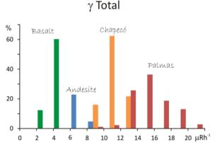
**Figure 14.** Total gamma-ray frequency ( $\mu Rh^{-1}$ ) histograms for the different volcanic rock types of Serra Geral Formation.
