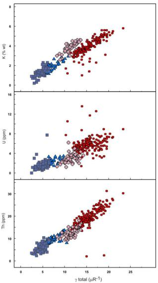
**Figure 15.** Total gamma-ray (γ total) vs K (% wt), U(ppm) and Th (ppm) obtained by gamma gamma-ray spectrometry during the field work. Legend: square= basalts, triangle= andesites, circle= ATP rocks, cross= ATC rocks.
