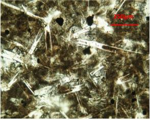
**Figure 3.** Photomicrography of ATP rock showing quench textures: hollow and swallowtail in microlites of plagioclase.
