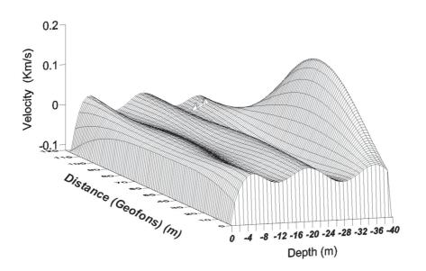
FIGURE 7. Perspective view of the mean seismic section.
