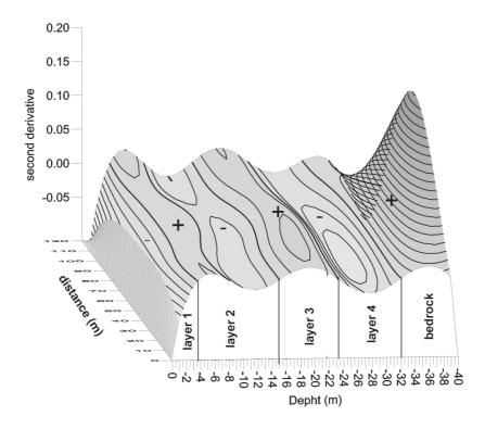
**FIGURE 8.** Perspective view of the second derivative of the mean section and delimitation of the hypothetical thickness of compactness, where the iso-value curve of the second derivative is zero.
