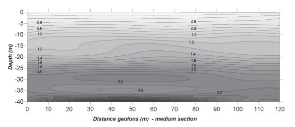
FIGURE 6. Mean seismic section showing velocities.
