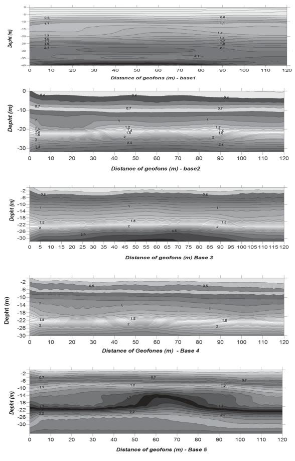
FIGURE 5. Seismic sections showing, in detail, the increase in wave velocity with depth.
